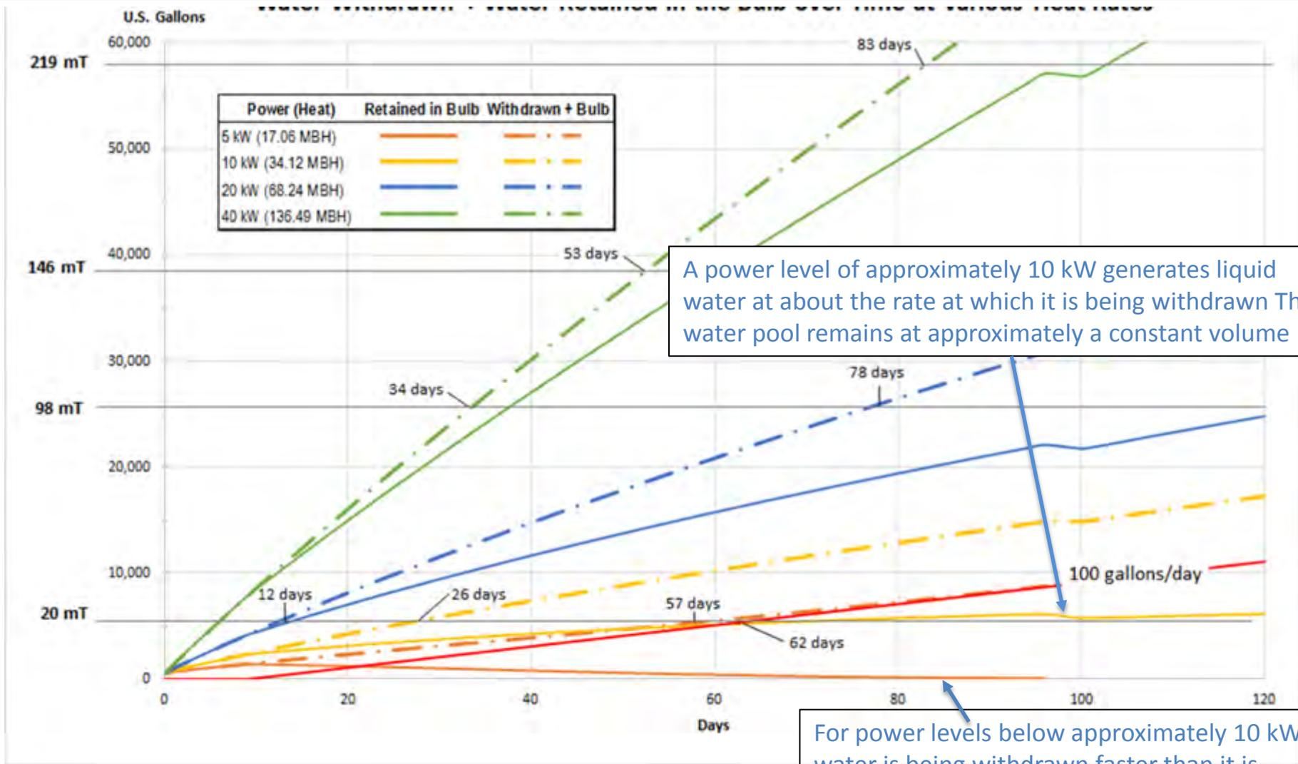
A power level of approximately 10 kW generates liquid water at about the rate at which it is being withdrawn. The water pool remains at approximately a constant volume.
